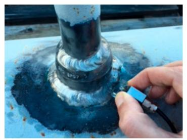
Manual scanning of nozzle welds is challenging
